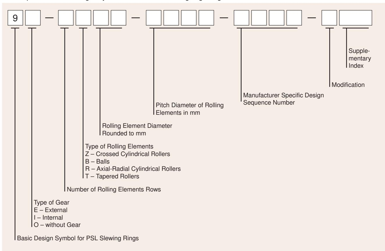
The designation is located on a non-functional surface of the slewing ring. It is made either electrochemically, or by stamping, or marked on a label fastened to the slewing ring.
