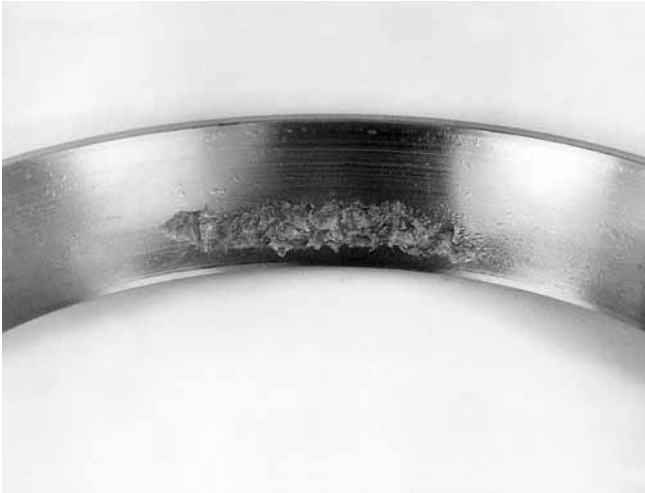
Fatigue of tapered roller bearing raceways - pitting. The pitting location is proof of a large edge load possibly due to misalignment of the surfaces.
