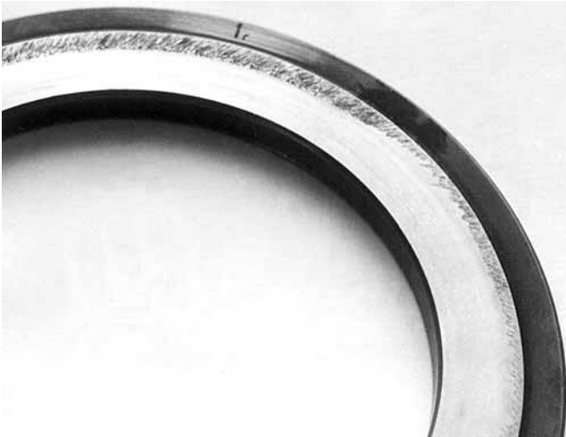
Seizing of guiding surface of a loose rib.
