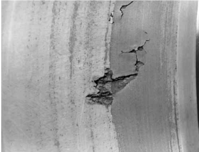
A detail picture of a cylindrical roller raceway fatigue - surface spalling due to an unsuitable lubricant.
