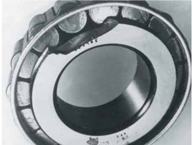
Chipping of a rib of a tapered roller bearing due to non-professional mounting.
