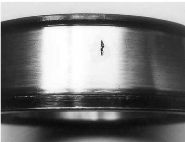
Fatigue of tapered roller bearing raceways - the initial and developed stage of pitting.
