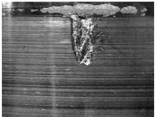
Craters and slipping marks on the raceway.
