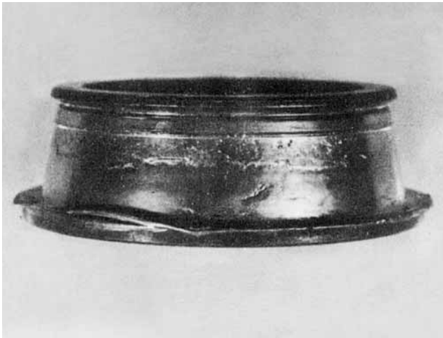
Deformation, or re-forming of the raceway and the supporting face of the inner ring of a tapered roller bearing due to the axial overload or insufficient lubrication.
