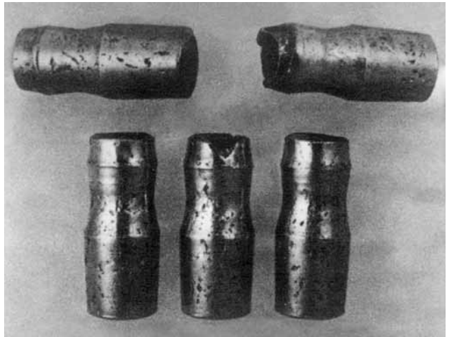
Deformation a spherical roller bearing rolling elements due to the axial overload or insufficient lubrication.
