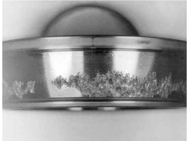
Fatigue of tapered roller bearing raceways - pitting. The pitting location is proof of a large edge load possibly due to misalignment of the surfaces.
