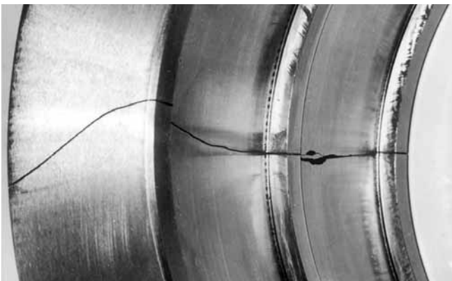
A cross crack in place of an insufficient leaning of the cylindrical roller bearing outer ring.
