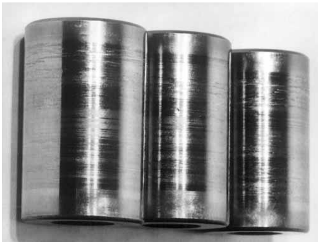
Seizing of cylindrical rollers on the rolling surface.
