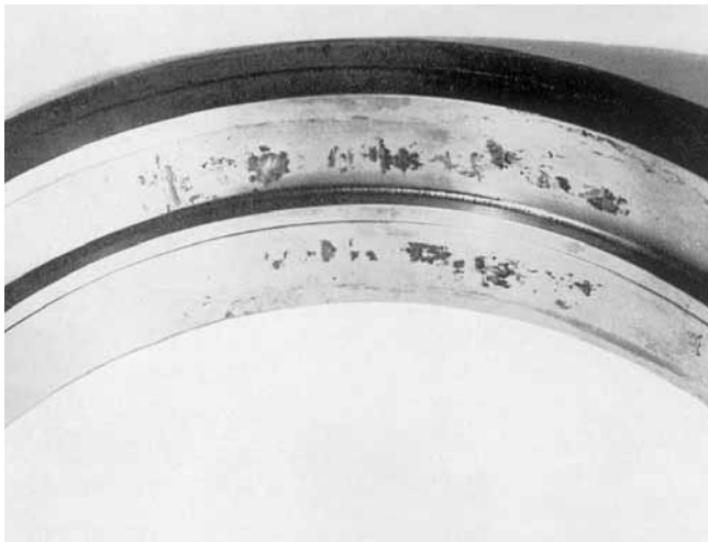
Chemical corrosion of an outer bearing ring raceway.
