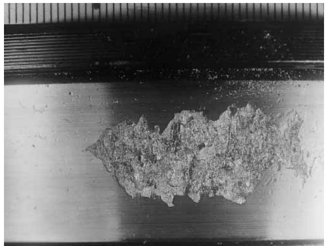
Fatigue of tapered roller bearing raceways - pitting. The pitting location is proof of a large edge load possibly due to misalignment of the surfaces.
